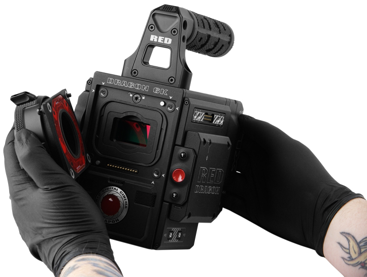
Figure: Remove the Lens Mount
