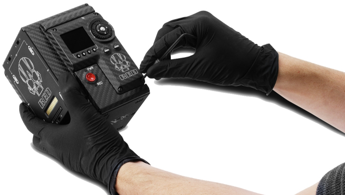
Figure: Reinstall the Side Module/Panel
