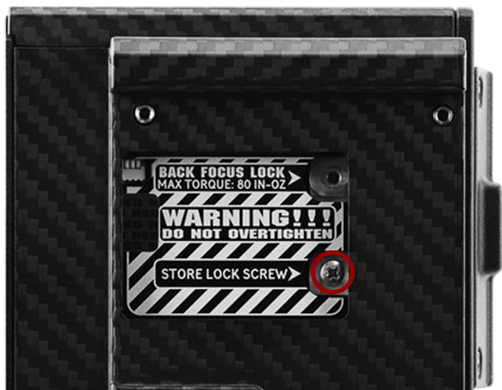
Figure: Remove Screw from Store Lock Screw Position
