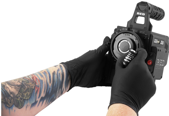
Figure: Remove the Lens Mount Screws
