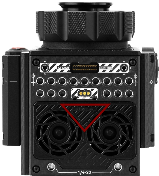
Figure: Do Not Obstruct WiFi Antenna
