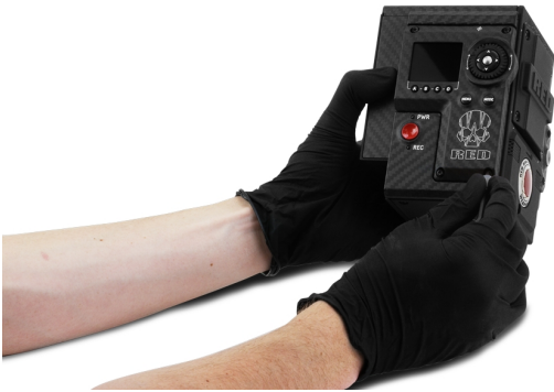
Figure: Remove the Side Module/Panel
