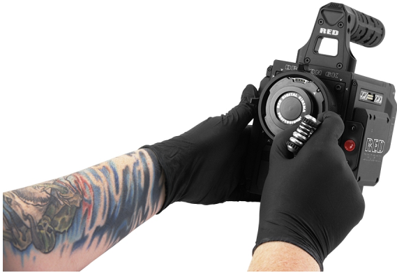
Figure: Remove the Lens Mount Screws
