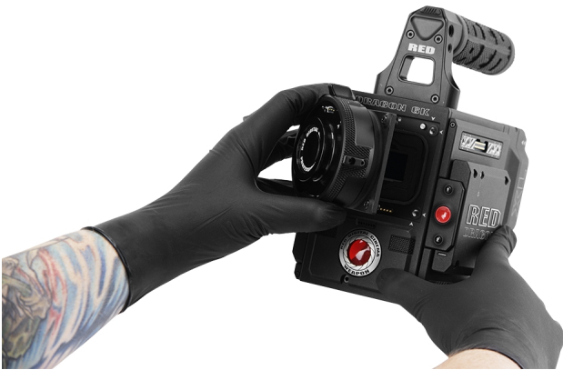
Figure: Align Lens Mount Pins
