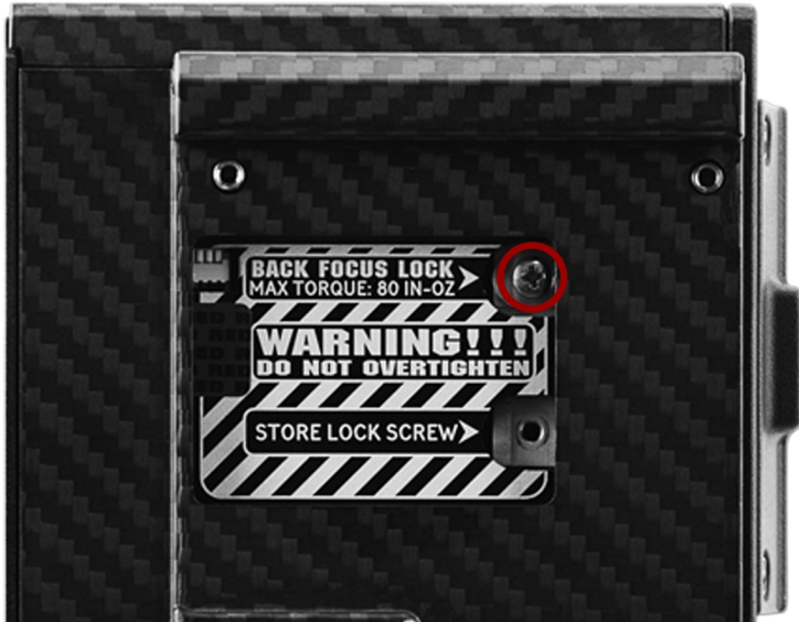
Figure: Back Focus Successfully Locked
