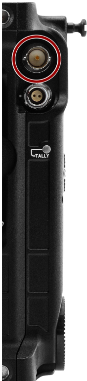
Figure: Front Face of the EVF male BNC Connector (looking at the front of the camera).
