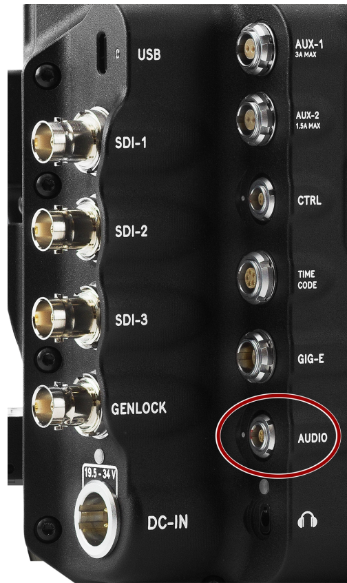
Figure: Front face of the female 5-Pin 00B audio connector (looking at the back of the camera).
