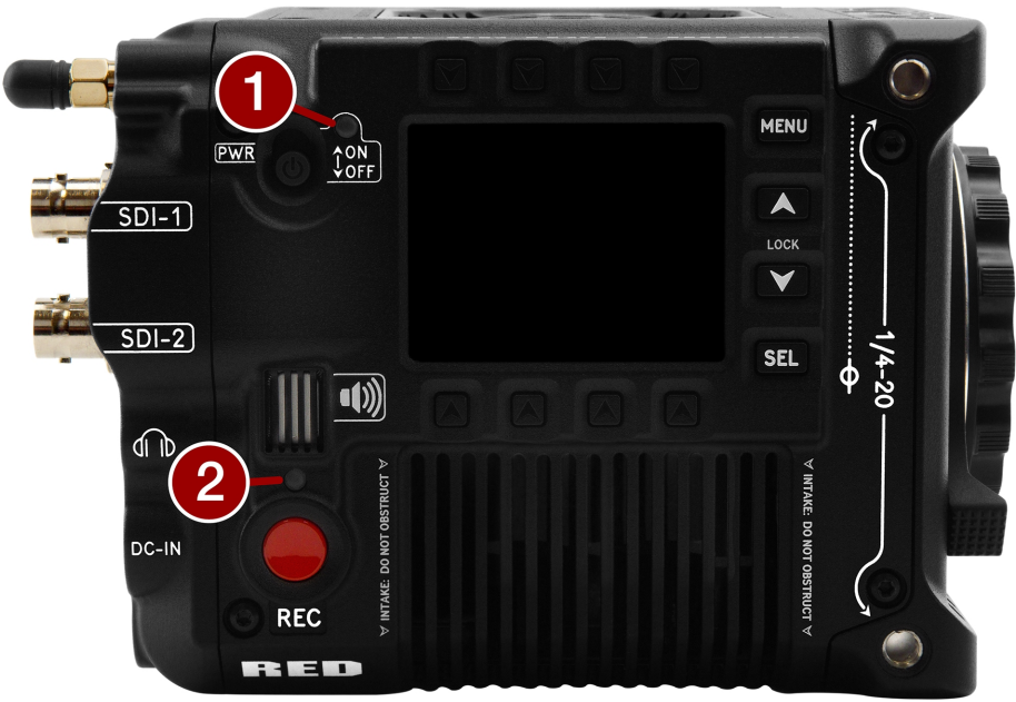
Figure: Camera LEDs, Right Side
