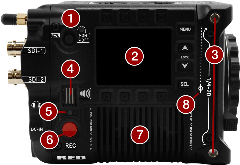
Figure: Camera Body Right Controls and Features
