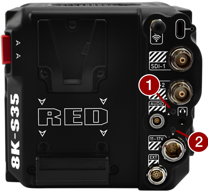
Figure: Camera, Back LEDs
