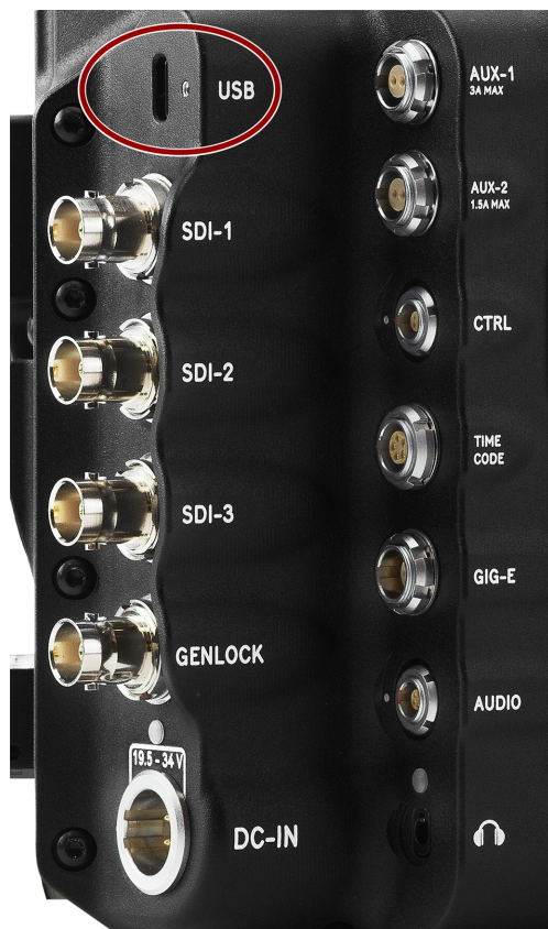
Figure: Front Face of the USB-C port (looking at the back of the camera).
