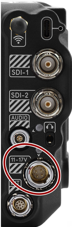
Figure: Front face of the male 6-Pin 1B DC power input connector (looking at the back of the camera).
